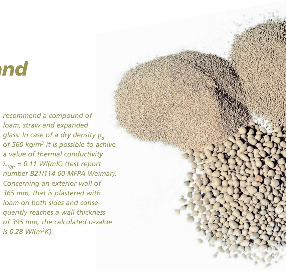
recommend a compound of loam, straw and expanded glass: In case of a dry density  $\rho_d$  of 560 kg/m<sup>3</sup> it is possible to achieve a value of thermal conductivity  $\lambda_{10tr} = 0.11 \text{ W/(mK)}$  (test report number B21/114-00 MFPA Weimar). Concerning an exterior wall of 365 mm, that is plastered with loam on both sides and consequently reaches a wall thickness of 395 mm, the calculated u-value is 0.28 W/(m<sup>2</sup>K).
